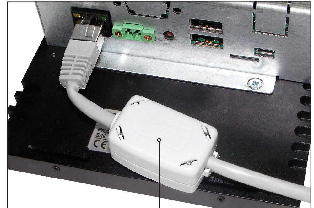
Meegeleverde openklapbare ferrietkern
